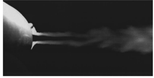
FIG. 2. Photograph of a jet. Smoke particles injected into the turbulent zones show an intense mixing and thus a visualization of the turbulent domains. Hardly any transport of smoke into the laminar core region takes place. Therefore, in a plane jet the core can clearly be detected photographically. Its parabolic time-averaged profile becomes transparent when the photographic exposure time is high.
